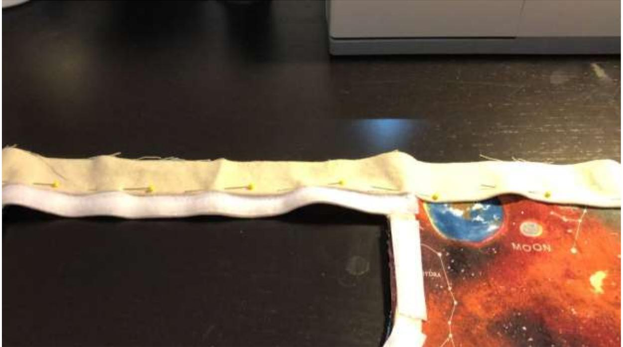
13. Sew together along the length of piece 1, again backstitching at the corners of piece 2 and 3, as this is a stress point.
